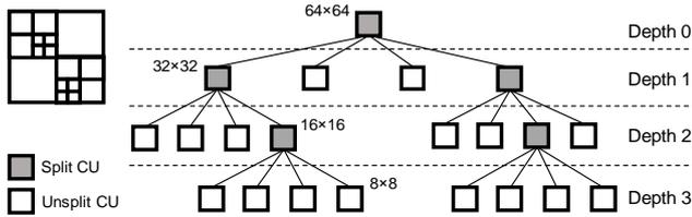
Fig.1: Example of a CTU partitioned into several CUs following the HEVC quadtree structure.
