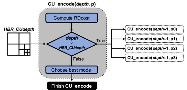
Fig. 3: CU splitting process using side information from decoder.
