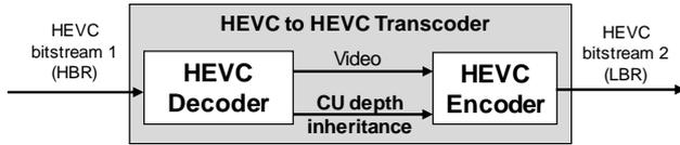
Fig. 2: CU splitting process using side information from decoder.
